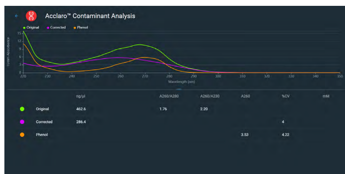
Figure 1: Acclaro contaminant analysis technology screen outlining the original concentration, corrected dsDNA concentration, and the absorbance contribution of phenol contamination. The original spectrum is shown in green, the corrected spectrum is shown in pink, and the phenol spectrum is shown in orange.
